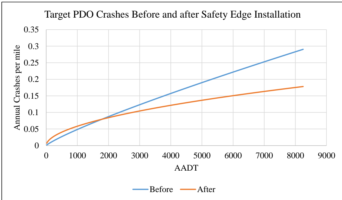
Figure 6. 7. Graph for Annual Target PDO Crashes per Mile Before and After Installation
